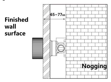
2. Mount the mixer body in place, connect the water supply and water outlet. To ensure there are no leaks, test the connection and check that the mixer body is level. Do not remove the plastic cover until the final fit-off.
